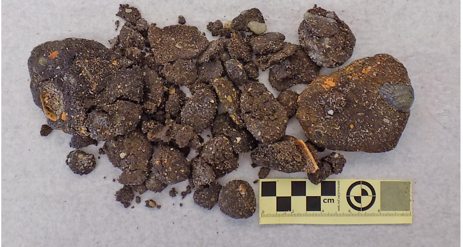
FIGURE 2. Surface residual balls from the Deepwater Horizon oil spill that scientists have found are mostly made up of pieces of sand, shell, and other materials and were loosely bound by oil containing various petroleum chemical such as polycyclic aromatic hydrocarbons. These samples were collected from Little Lagoon Pass, AL, on July 19, 2015 by Professor Clement at Auburn University. (P. Clement, Auburn University photo)
