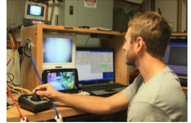
FSU PhD student Chris Malinowski flies the MILET 2-3 m above bottom by reeling cable in or out from the winch.
