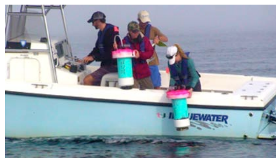
CARTHE scientists releasing SCOPE drifters just outside the surfzone. (Photo provided by CARTHE)
