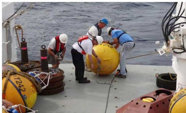
A team prepares to deploy a series of anchored moorings. The connecting lines secure the instruments that record data such as temperature, pressure, and velocity.
