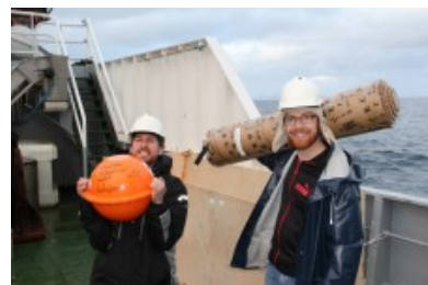
Kai H. Christensen (R) and Johannes Rohrs (L) prepare to deploy two types of surface drifters. The drifter in the cardboard box unfolds once in contact with water. (Photo by: Göran Broström)
