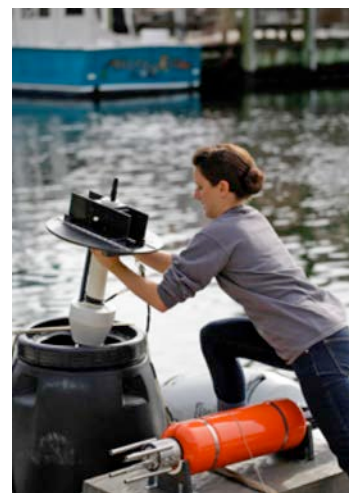
Kimberly Arnott (Texas A&M University, Corpus Christi) prepares microstructure instruments for deployment to record measurements of water turbulence such as dissipation and diffusivity. (Photo provided by CARTHE)
