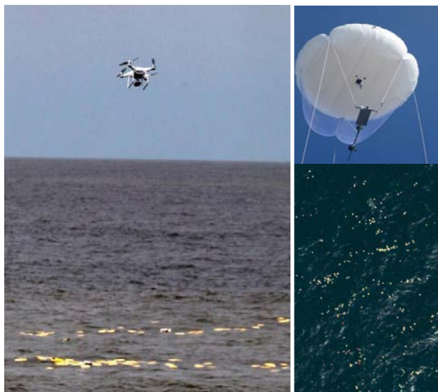
FIGURE 7. (left) Drone monitoring a patch of drift cards during an experiment examining the near-surface layer of the ocean; (right top) high-resolution camera system hanging from the aerostat; (right bottom) image from the aerostat camera of thousands of drift cards gathering into lines during a dispersion experiment. Courtesy of CARTE
