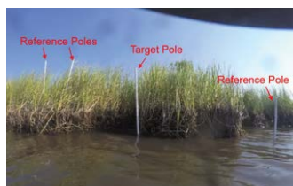
FIGURE 8. Researchers documented daily marsh loss using PVC poles and time lapse photography. Video ( https://www.youtube.com/watch?v=bEumDAFWnqW ) shows a time lapse of land loss in coastal Louisiana. Courtesy of CWC/ Giovanna McClenachan
