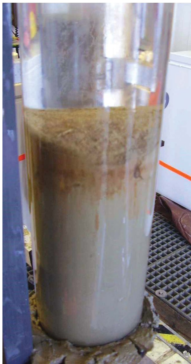
FIGURE 1. A layer of marine oil snow covering seafloor sediments in a core sample collected during a November 2010 cruise at a site 175 kilometers (km) east, northeast of the DWH wellhead in 400 meters (m) water depth (site MC04). Courtesy of Patrick Schwing, University of South Florida, College of Marine Science
