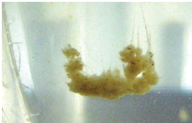
FIGURE 8. Close-up shot of a marine oil snow particle formed in the laboratory. Courtesy of Uta Passow/ECOGIG and Aggregation and Degradation of Dispersants and Oil by Microbial Exopolymers (ADDOMEx, http://www.tamug.edu/addomex/ ) research consortia
