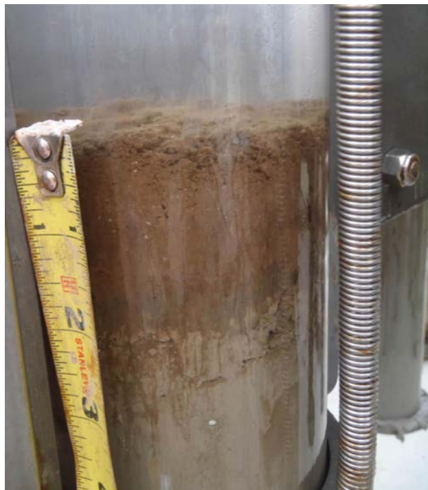
FIGURE 9. A thick, fluffy floc layer sampled from the seafloor, as observed in a sediment core taken in the Gulf of Mexico. Photo taken in September 2010. Courtesy of ECOGIG/ Samantha Joye
